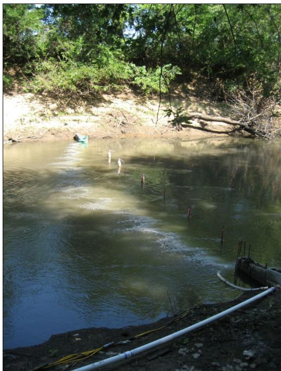
**Figure 4.** Image of the sound-bubble-strobe light barrier operating in Quiver Creek, Havana, Illinois, USA. Photograph by Blake Ruebush.
