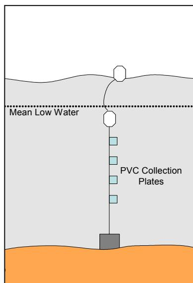
**Figure 4.** Schematic diagram of collector deployment. Collector size was 10 cm × 10 cm.
