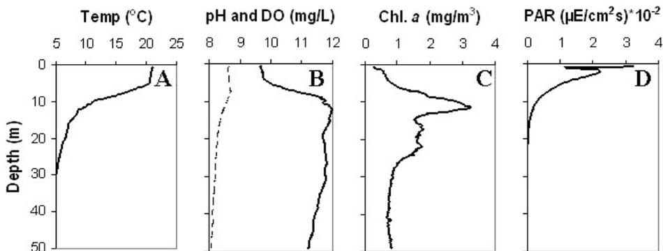
**Figure 3.** Vertical profiles of selected limnological parameters at station 2 on 18 June 2007: temperature (A), dissolved oxygen (DO: B, solid line), pH (B, dashed line), Chl. *a* (C), and photosynthetic active radiation (PAR: D). Conditions shown are typical of profiles during summer at all stations.
