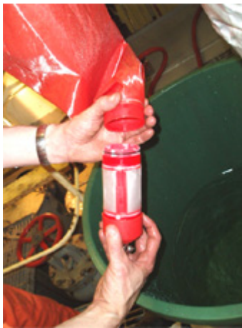
Figure 4. Cod-end may be unscrewed from filtering bag
