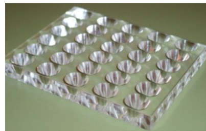
Figure 5. Newly designed zooplankton counting chambers
